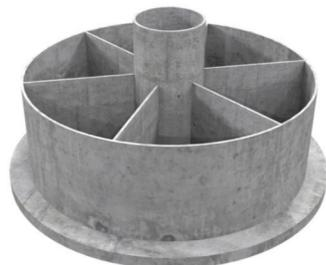
The main structure is mostly made with cast-in-place concrete, with the following elements: slab, perimeter wall, bulkheads (6x) and central tube. The cells are filled with XPS foam blocks and ballast tanks.
