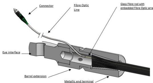
The composite material is bonded together at the terminals with an advanced resin system which also act as load transmitter from the structural rods to the terminals.
