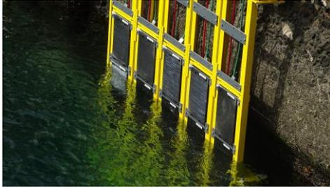
This fact has made possible to select the most suitable additives combinations for the full antifouling and anti-bite evaluation, that is being carried out following a methodology based on the standards ASTM D3623 and ASTM D6990.
