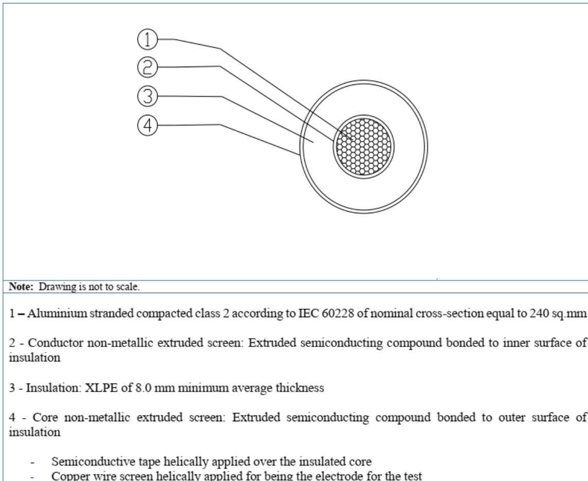
Figure 1. Cable structure
