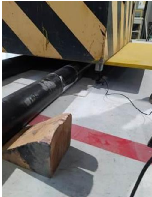
Figure 7. Crush test for long term
