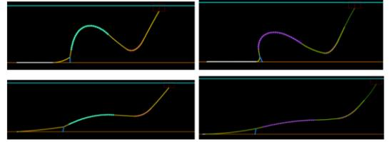
This numerical model will provide with tensions and curvatures to the developer of the power cable.
