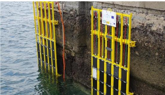
Different plastic materials have been developed for mooring cables, power cables and floater. The methodology based on the standards ASTM D3623 and ASTM D6990 and the design of the experiments have allowed us to select the most suitable antifouling and anti-bite additives, which are being evaluated in real sea conditions.
